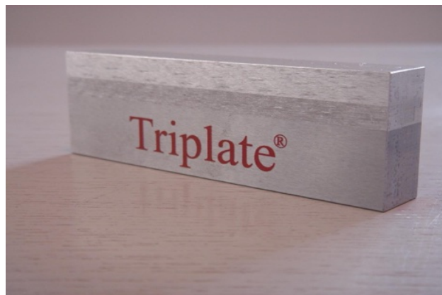
Figure 1. Triplate® transition joint, three-layer composite strip (steel / Al 99.5% / AlMg4.5Mn). The three layers are visible on the end face.
