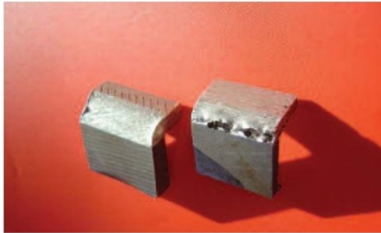
Figure 5. The consequences of the Hammer Bend Test (MIL-J-24445A). Left: vacuum-clad Triplate®: interface intact, no defect formation. Right: open-air cladding: oxide conglomerates open out visibly at the turbulent transition layer. Source: Buijs, N.W. (2010). Explosive Welding of Metals in a Vacuum Environment. Stainless Steel World, March 2010. (Photo: Innomet b.v.)
