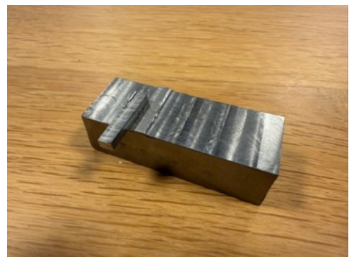
Figure 9: Perfect shear-test. Fracture in the flyer-material. 490Mpa, Alloy 625 clad
