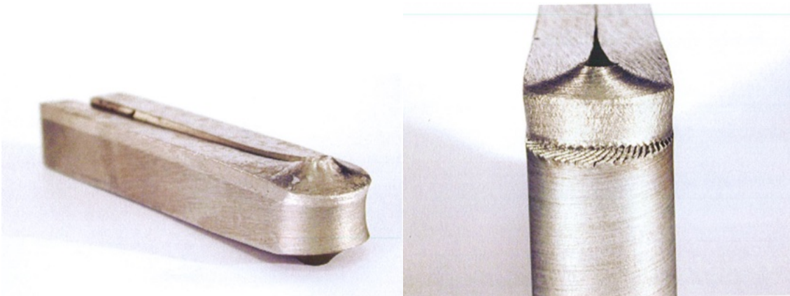
Figure 11: Vacuum cladding vs. open-air/atmospheric cladding side-bend-test.
